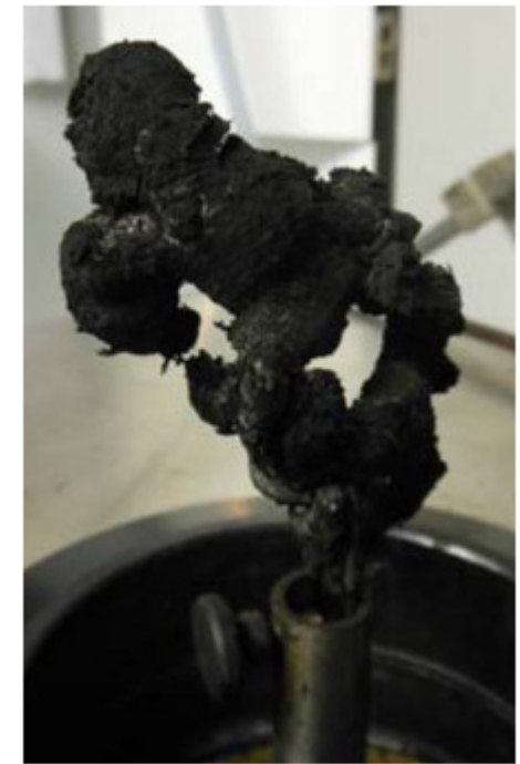
Picture of p(P-pPDA) burned in a rich oxygen atmosphere (38.5%)
